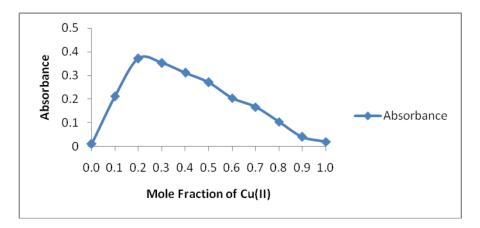
Figure 4: Job's plot for Cu(II)-NH<sub>3</sub> complex
