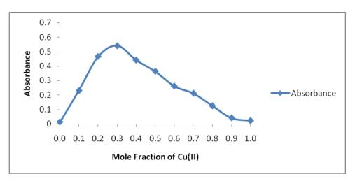
Figure 17: Job's Plot for Cu(II)-N-Propanoyl L-Phenylalaninol complex
