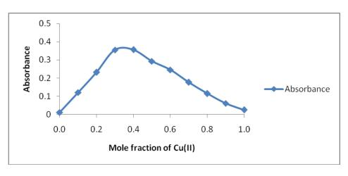
Figure 7: Job's Plot for Cu(II)-Ethanolamine Complex
